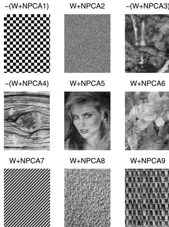
Fig. 12.6 The separated images using the nonlinear PCA criterion and learning rule.
