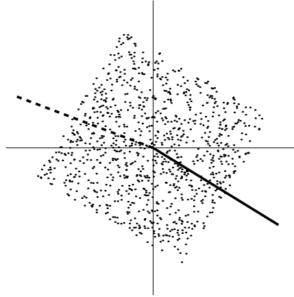
Fig. 8.16 Result of FastICA using kurtosis, for ICs with uniform distributions. Dashed line: w after the first iteration (plotted longer than actual size). Solid line: w after the second iteration.
